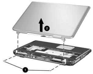
Removing the Display Assembly
